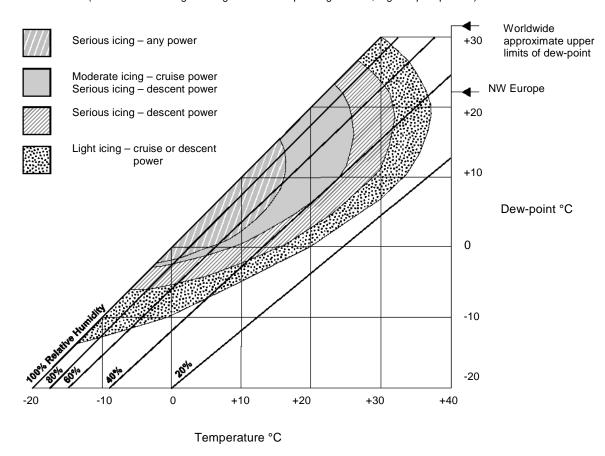
3.5 Impact icing occurs when flying through snow or sleet, or in cloud in which super-cooled water droplets are present. It can occur, but is less frequent, when flying through super-cooled rain or on an aircraft which has a surface temperature below 0° C when through rain which is above freezing temperature. The ambient temperature at which impact ice may be expected to build up most rapidly is about -4° C in conditions in which visible ice is forming on other parts of the aircraft.
