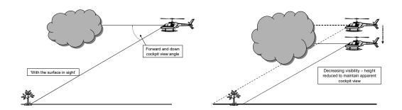
Such descent, if undetected, could obviously lead to dangerous situations developing in terms of CFIT or collision with an obstacle. In addition, the increased perception of ground speed at lower height could lead to an inadvertent reduction in airspeed and hence more height loss and reduced stability.
