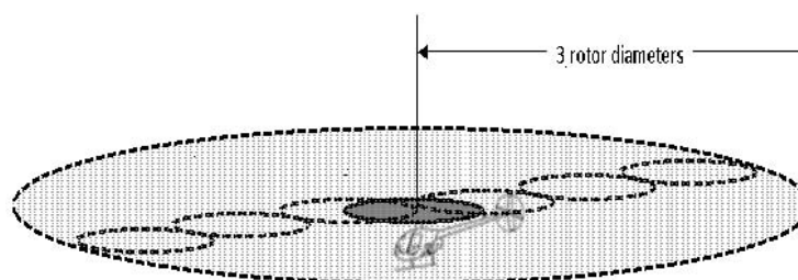
Figure 17*: Helicopter hover or slow hover taxi, 3-rotor diameter avoidance area.
